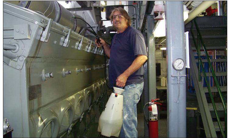
Luhr Bros. engineer degreases diesel engine.
